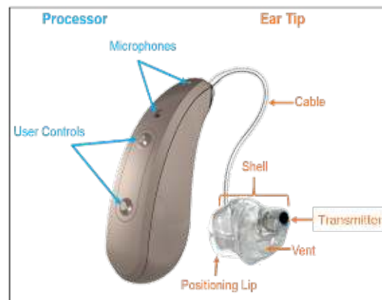
Figure 3. Earlens Processor and Ear Tip
